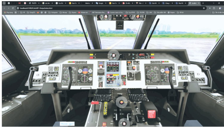
Figure 5. Virtual Cockpit Explorer displaying panoramic cockpit view with interactive hotspots for accessing related documents, 3D models, and videos
